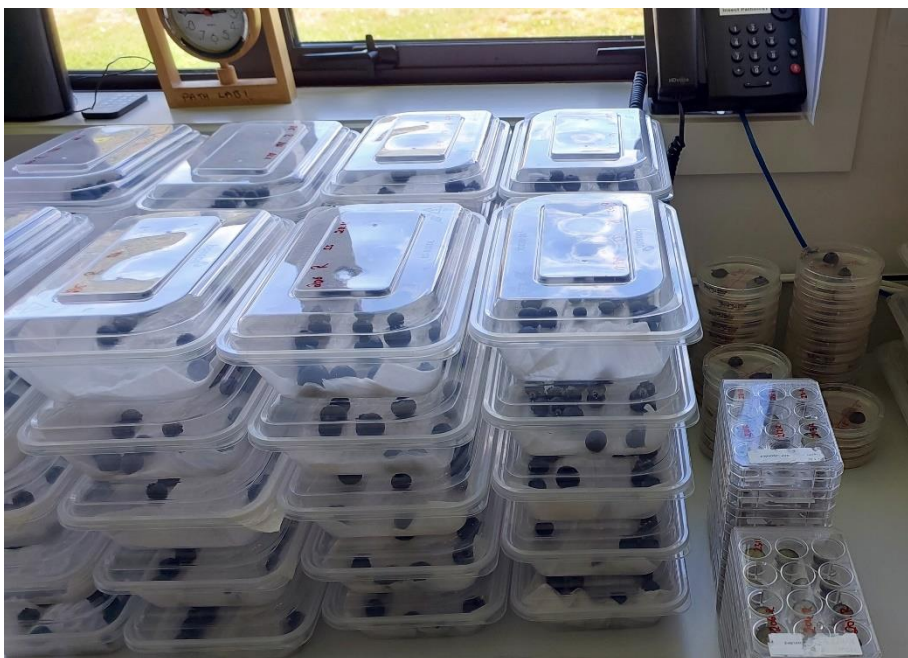
Figure 3.1. Humidity chambers with surface sterilised and non-surface sterilised blueberry fruit, titre plates with surface-sterilised fruit, and agar plates with surface-sterilised fruit.
