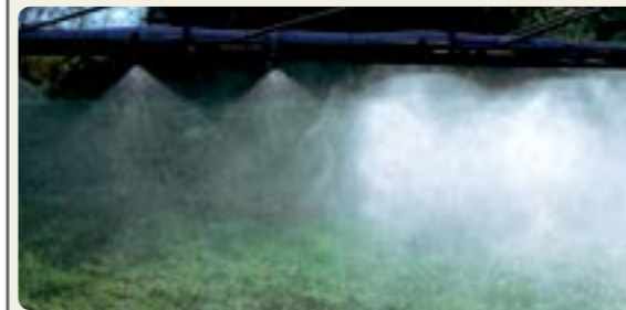
Figure 3 Coarse spray droplets (left) produced with a TurboDrop® nozzle, compared to fine droplets (right) produced with a conventional XR TeeJet® nozzle.
