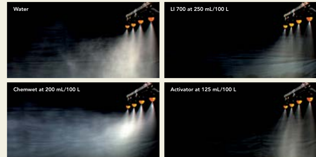
Figure 118 XR TeeJet®110-02 nozzle type sprayed at 2.5 bar
