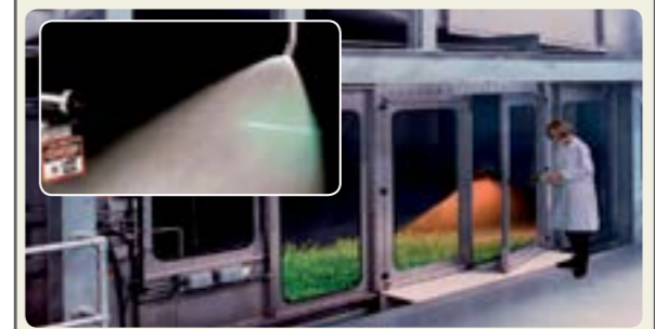
Figure 4 Wind tunnel in Silsoe, England (Pictured inset: Laser measurement)
